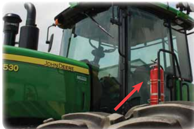
Notice the proper location of this fire extinguisher on a tractor.
